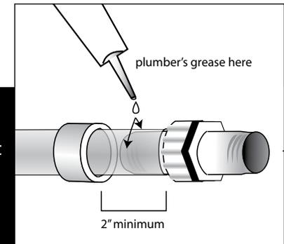
Holding ProPEX ring, insert female fitting, pushing & wiggling hose from side to side until hose end is half the width of the ring from the fitting's shoulder.
