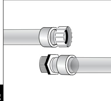
ProPEX ring needs to overlap fitting so that the tapered end of the fitting is visible beyond the ring.
